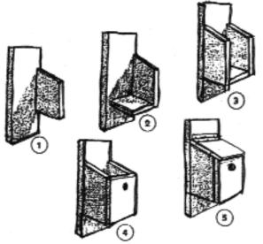
The entrance hole should be no less than 125mm from the floor level
